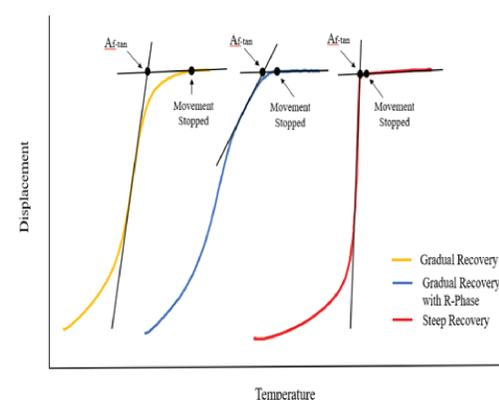
Figure 2. Displacement vs. temperature curves showing gradual and steep recovery
