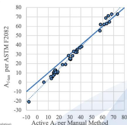
Figure 1.  $A_{f-tan}$  per ASTM F2082 plotted vs. Manual Method
